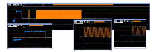
In this example 4 timing windows are being displayed. Window 1 is showing the entire buffer. Window 2 is showing a zoomed in section around the trigger (Red cursor) event. Windows 3 and 4 are each showing a different part of the waveform and are zoomed differently.
